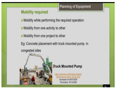
So, the next important factor is it the mobility required. So, it depends upon the project additional actual activity. So, what is your mobility required with respect to equipment during the particular activity? Or what is the level of mobility needed to move the equipment from one activity to another activity? Or what is the level of mobility needed to move the equipment from one project site onto the project site?
