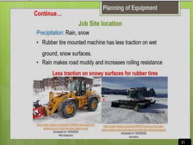
So, in some places you can see that for most of the months there will be continuous heavy rainfall. So in those places obviously the terrain will be very poor like it will be having the poor underfoot conditions with a very high rolling resistance the terrain will be very muddy. So, as
