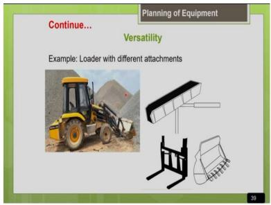
So the next one is the front end the loader, you can see the loader with the different attachments. Just for different applications you can change the attachments and make it more versatile. So you can see the loader with the front end bucket here. So as everyone knows, the loader can be used as a hauling equipment for a very short distance of say, up to 100 meters and it is good at excavating material at or above the ground level.
